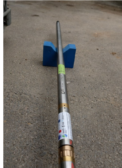
Robertson Geologging probe for determination of seismic velocities in boreholes
