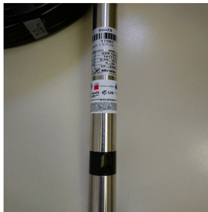
Temperature, electrical conductivity and groundwater level gauge
