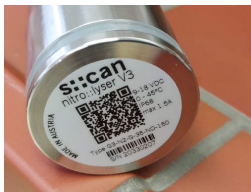
Scan Nitrolyser probe for measuring nitrate concentrations in groundwater
