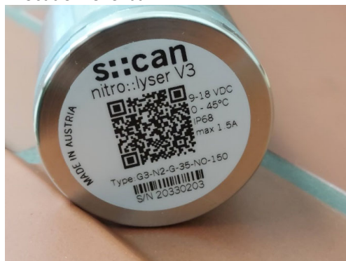
Scan Nitrolyser probe for measuring nitrate concentrations in groundwater
