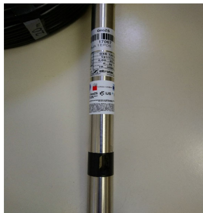
Temperature, electrical conductivity and groundwater level gauge
