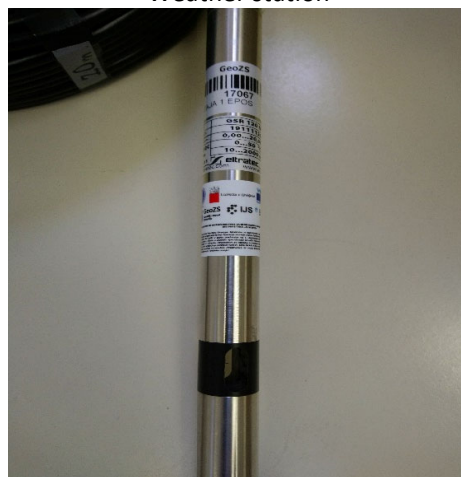
Temperature, electrical conductivity and groundwater level gauge
