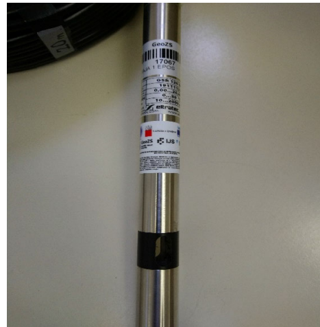
Temperature, electrical conductivity and groundwater level gauge
