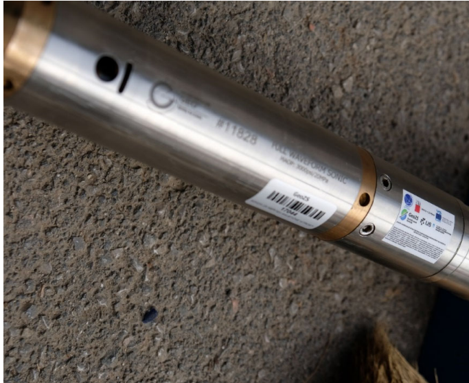
Robertson Geologging probe for determination of seismic velocities in boreholes
