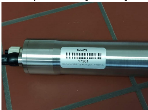
Scan Nitrolyser probe for measuring nitrate concentrations in groundwater
