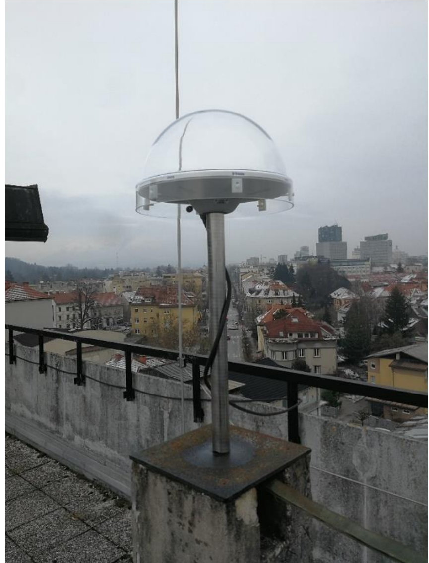
Figure 21: Trimble Zephyr 3 Geodetic GNSS antenna at GNSS station FGG300SVN
