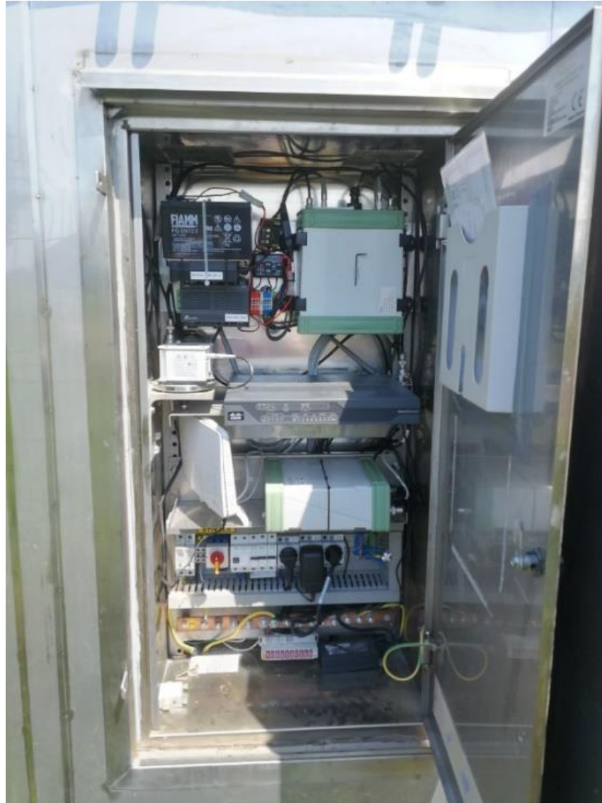
Figure 5: Leica GR30 GNSS receiver at the GNSS station PZA100SVN of the SIGNAL network (approximate position (ETRS89): \varphi = 45^{\circ} 35' 26.73'' \lambda = 15^{\circ} 15' 38.34'' h = 212.7 m)
