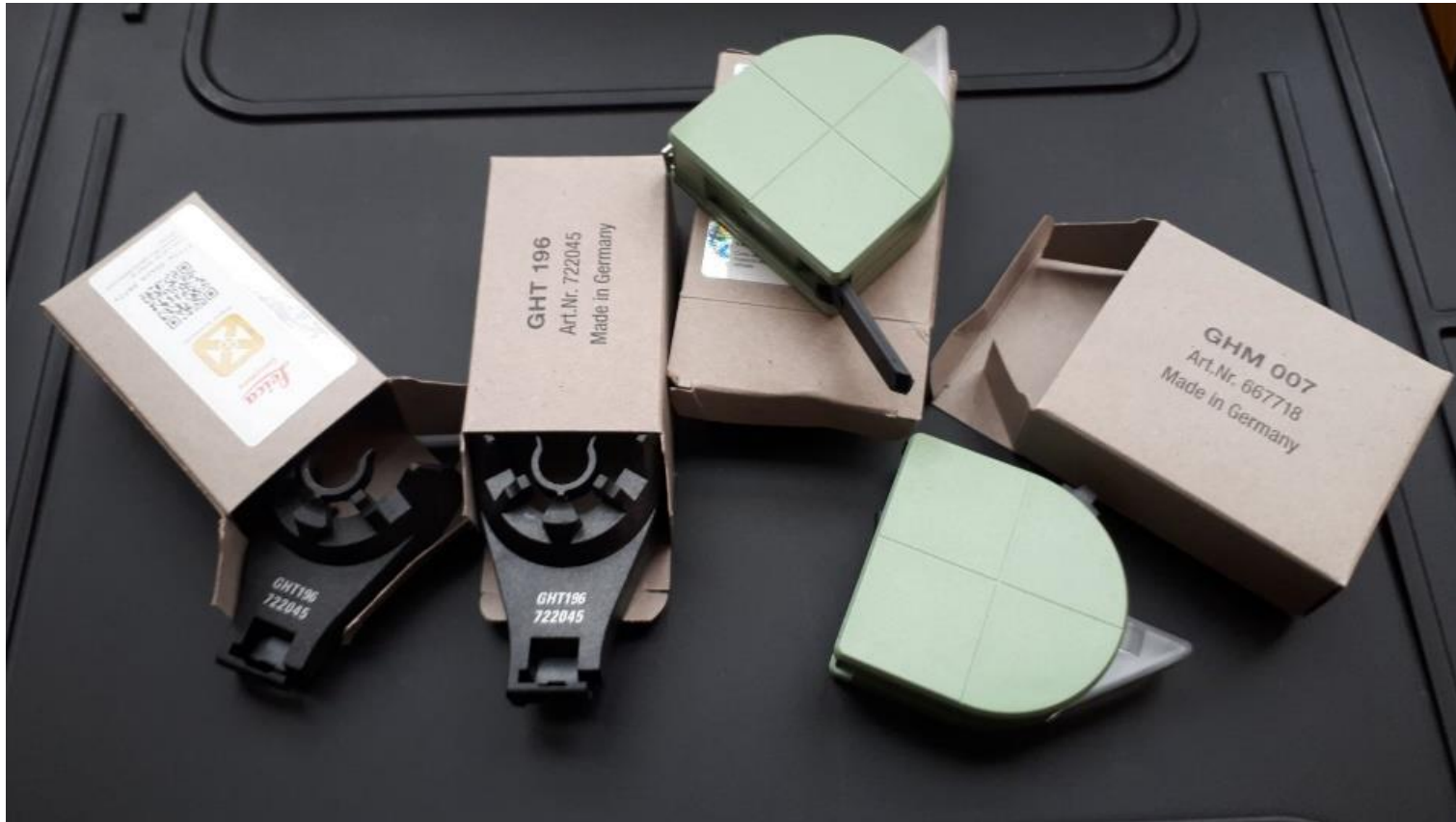
Figure 17: 2x Leica GHM007 instrument height meter with Leica GHT196 Tribrach distance holder
