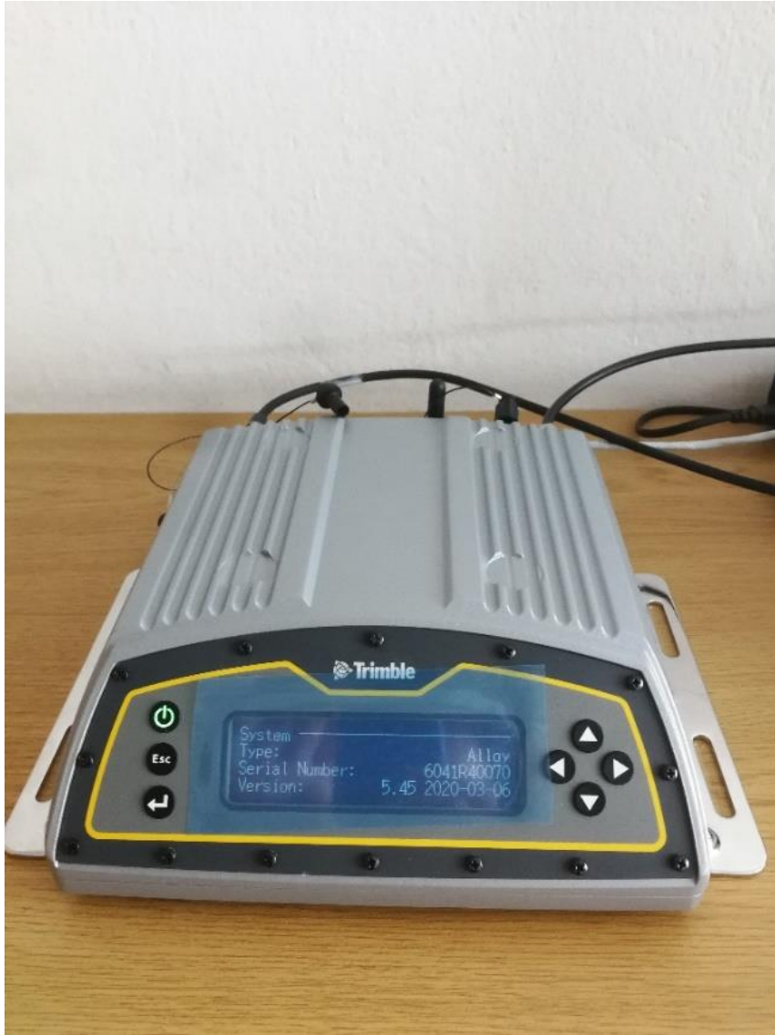
Figure 20: Trimble Alloy GNSS receiver at GNSS station FGG300SVN
