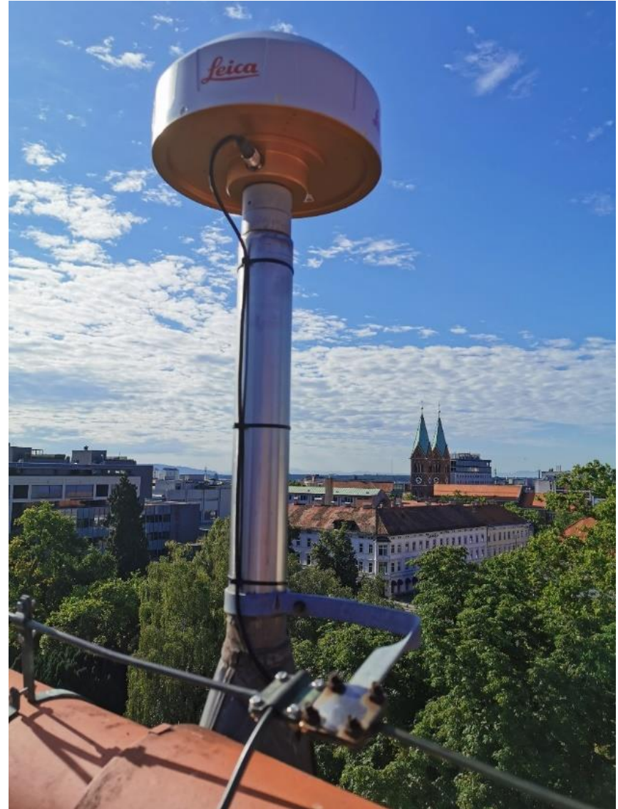
Figure 3: Leica GR30 GNSS receiver (left) and Leica AR20 GNSS antenna (right) at the GNSS station MRBR00SVN of the SIGNAL network (approximate position (ETRS89): \varphi = 46^{\circ} 33' 43.87'' \lambda = 15^{\circ} 38' 55.41'' h = 342.9 m)
