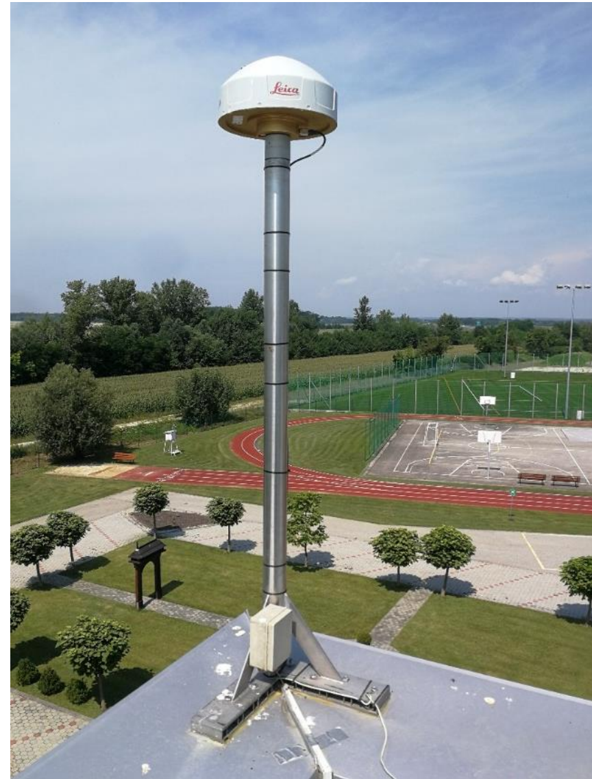
Figure 2: Leica GR30 GNSS receiver (left) and Leica AR20 GNSS antenna (right) at the GNSS station LEND00SVN of the SIGNAL network (approximate position (ETRS89): \varphi = 46^{\circ} 33' 53.00'' \lambda = 16^{\circ} 26' 49.57'' h = 219.9 m)
