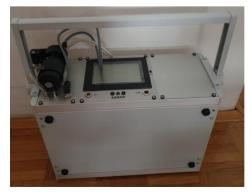
3. RTM 1688-2 – Radon and thoron monitor (Sarad, Germany) (one monitor)
