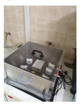
2. EQF3220 – Radon/Thoron gas & Decay Product monitor for attached and unattached decay products (Sarad, Germany) (one monitor)
